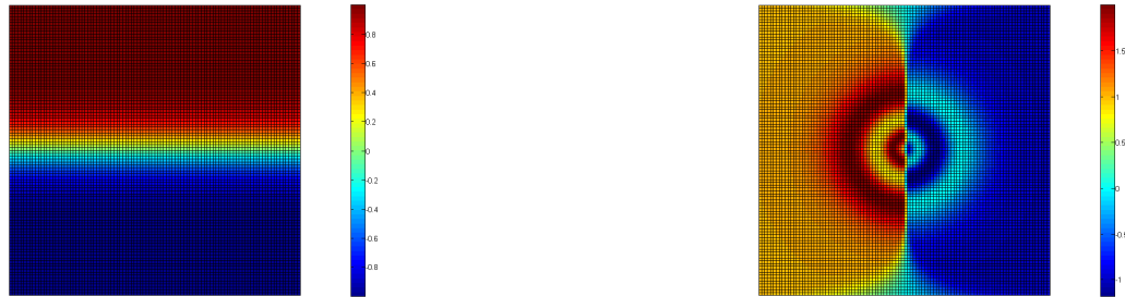
Figure 5.2: Doswell frontogenesis with source term: initial condition u_0 (left) and target function u_T (right),
