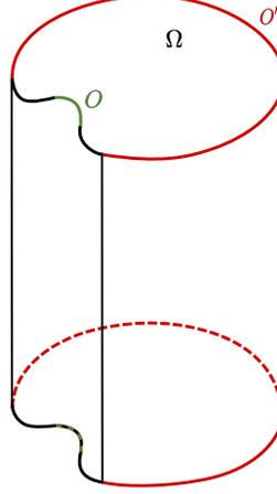
FIGURE 2. Cylindrical domain where waves evolve. In green the support of the source  $g$  to be identified, and in red the subset of the boundary where measurements are done.
