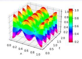
Figure 18: PINN-predicted solution to wave equation with Neumann boundary conditions
