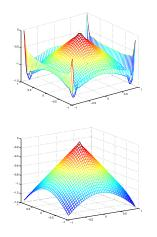
Figure: Orbital derivative of the Lyapunov function with respect to the original system using Algorithm 2 with 360 points(top), 1520 points (bottom).
