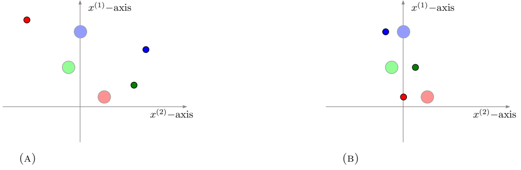
FIGURE 4.1. (A) Initial configuration for the simultaneous control before applying Theorem 1. The big colored circles represent the target locations for each point, denoted by small circles. (B) Configuration after controlling the x^{(1)} -component of each point.
