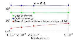
We observe that the control cost and the optimal energy remain bounded as  $h \rightarrow 0$ . Furthermore, we also see that the discrete  $L^2$  norm of the solution at time *T* behaves as *h*, which is the expected convergence rate. All these facts **provide numerical evidence indicating that the null controllability is fulfilled when** s = 0.8.
