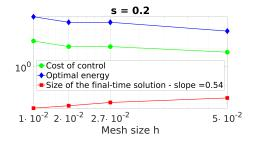
We observe that the discrete  $L^2$  norm of the solution at time T tends to zero as  $h \rightarrow 0$ , confirming computationally the approximate controllability of the equation.
